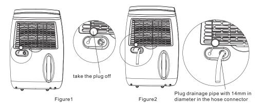
Note: Smoothly stretch the drainage, for if it is flat or twists together, drainage will not go on right; even the unit can not work normal. During the operation drainage pipe should never be in higher position than the hose connector.
